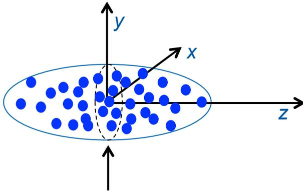
Particles close to the peak line density (often in the bunch center) will have the largest tune spread
