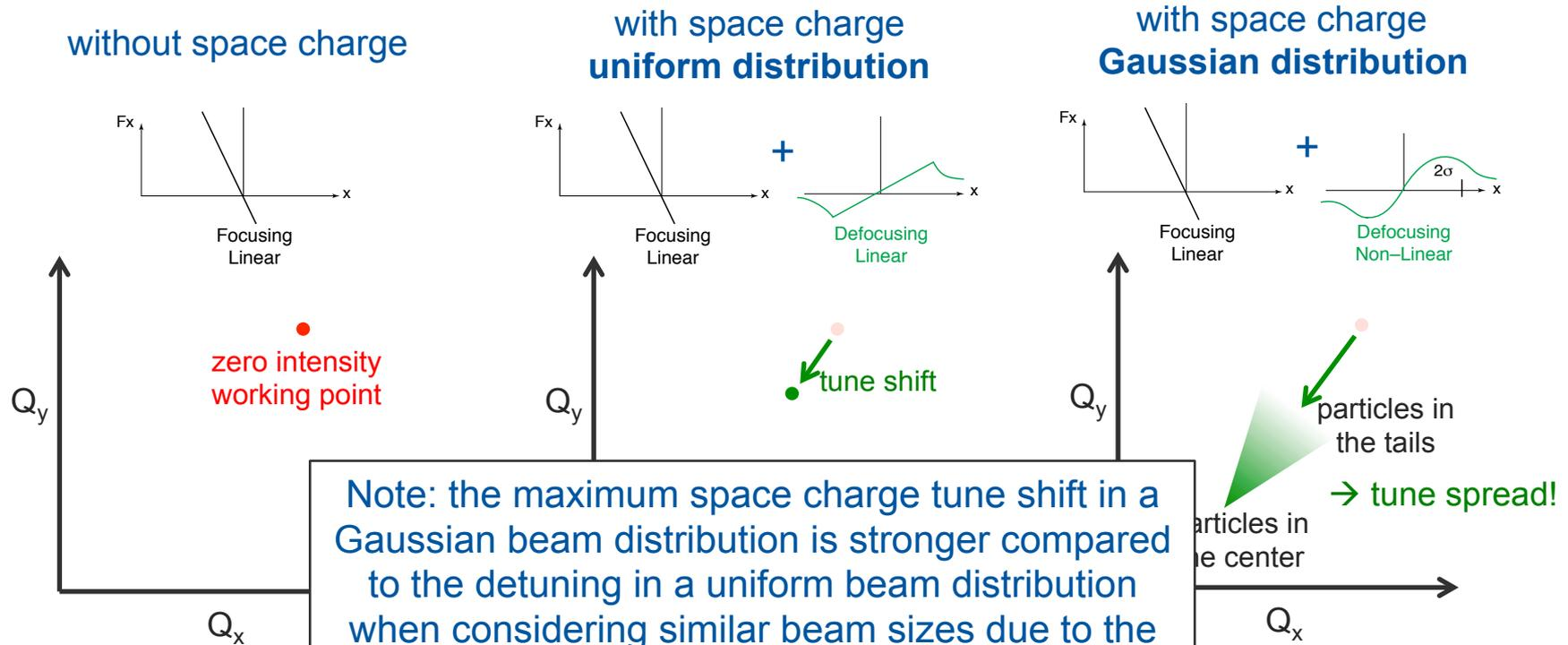
Note: the maximum space charge tune shift in a Gaussian beam distribution is stronger compared to the detuning in a uniform beam distribution when considering similar beam sizes due to the higher particle density in the beam core!
