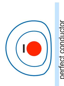
If the skin depth is very small (rapidly varying fields), fields do not penetrate and the magnetic field lines are tangent to the surface.
