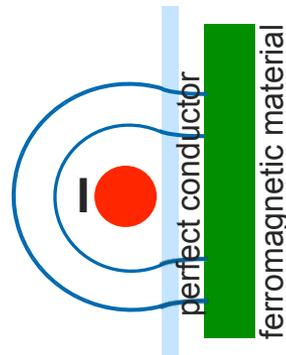
If the fields penetrate and pass through the vacuum chamber, they can interact with bodies behind the chamber
