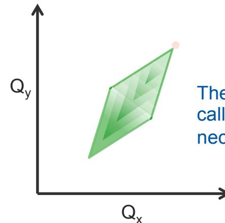
The tune footprint is also called the space charge necktie due to its shape
