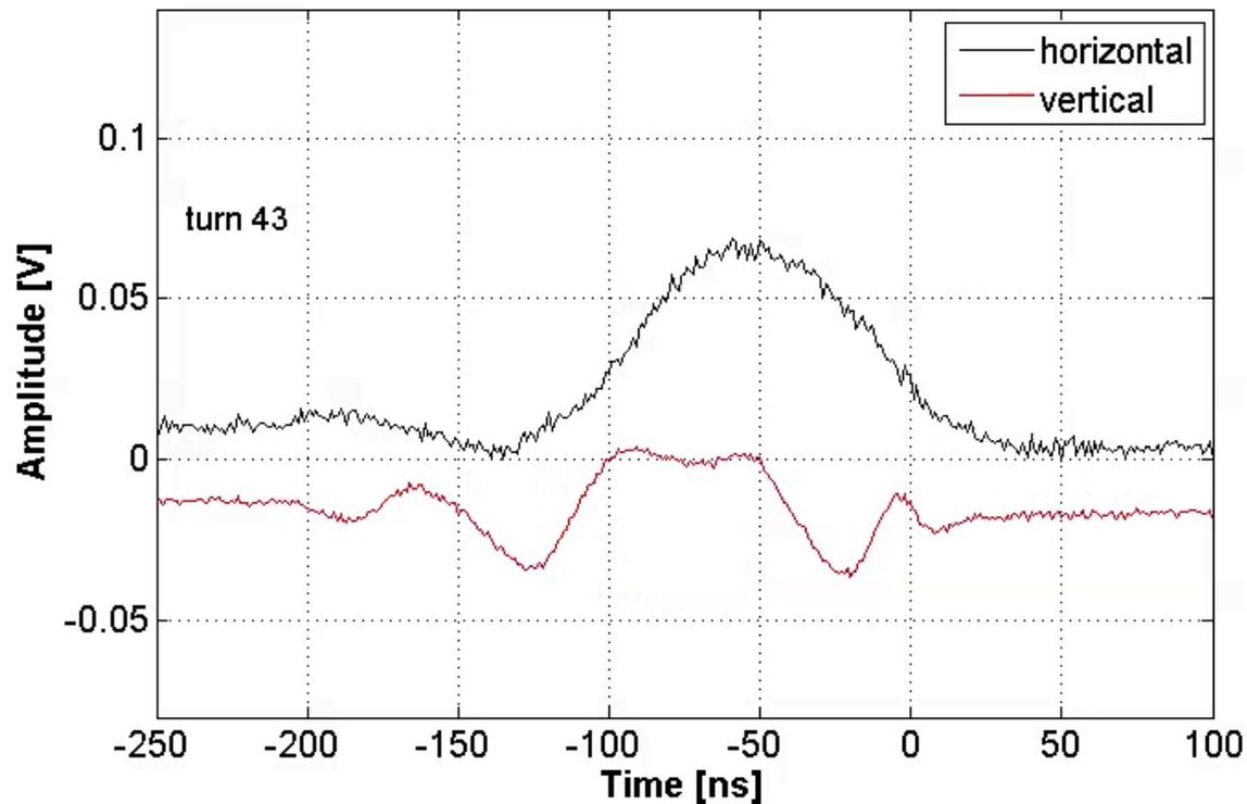
transverse position along the bunch measured with a wide-band pick-up (bunch length about 200 ns)
