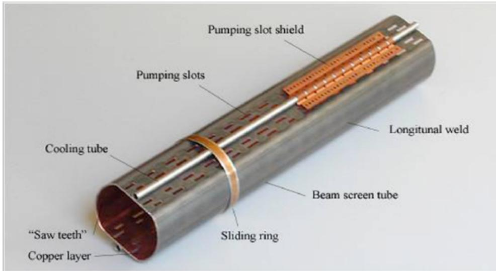
→ All along the arcs and in other cold regions of the LHC, a beam screen is interposed between the beam and the cold bore
