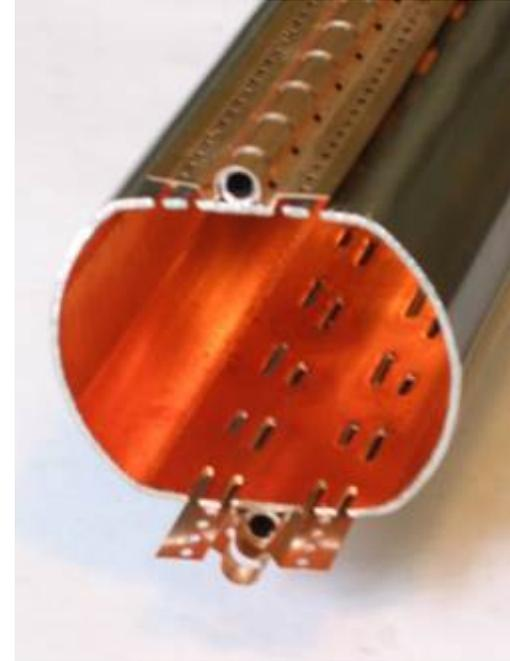
→ The impedance model includes the weld on one side of the beam screen, which means a small longitudinal stripe of exposed StSt, as well as the pumping holes
