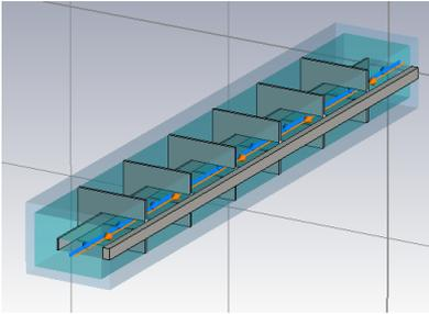
– Original kicker without serigraphy, typical broad-band behaviour, here some ringing is due to the longitudinal segmentation
